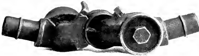
VIEW OF RADLEY'S AUTOMATIC OPENING ANGLE COCK AND HOSE COUPLING COUPLED UP.
